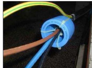
According to the "test" setup in this document, here is an actual picture of the cores this particular manufacturer used. As seen, there is no air space between cores and cabling. Also noticeable is the color and type of core. These cores are epoxy coated (lighter blue), and not in the blue case.
